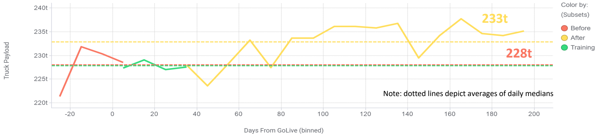
Figure 3 – Median Truck Payload per day sectioned into 'Before' and 'After' implementation of Titan 3330™ system.
